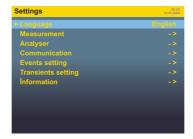
At main screen, move to parameter Settings to access device various configuration sub-menu. Some of the device parameters and functions can be enabled and configured only by PC and software.
